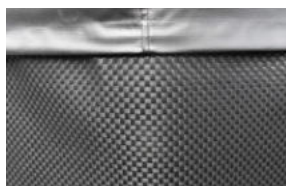
Exterior casing in braided PVC
